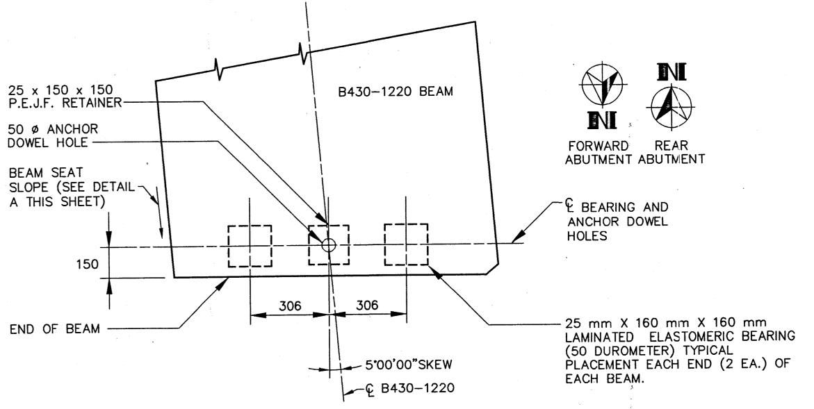
ANCHOR DOWEL AND BEARING PAD LAYOUT (REAR ABUTMENT SHOWN)
