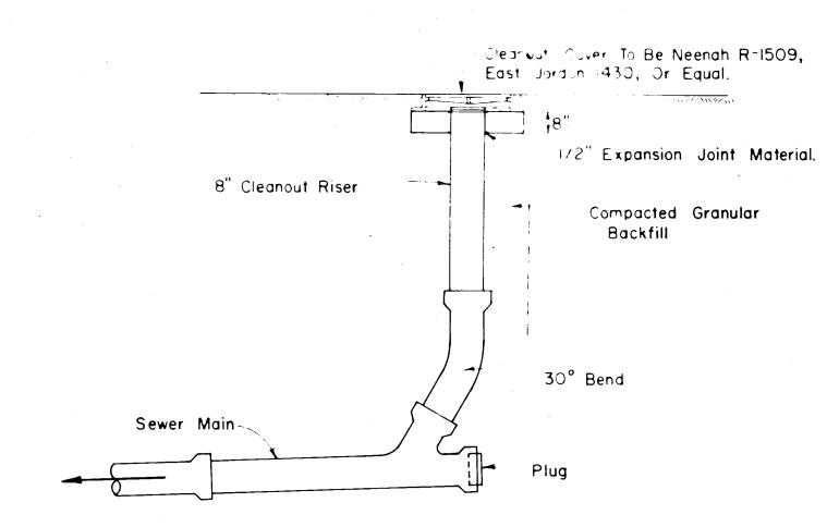
GRAVITY SEWER CLEANOUT DETAIL
