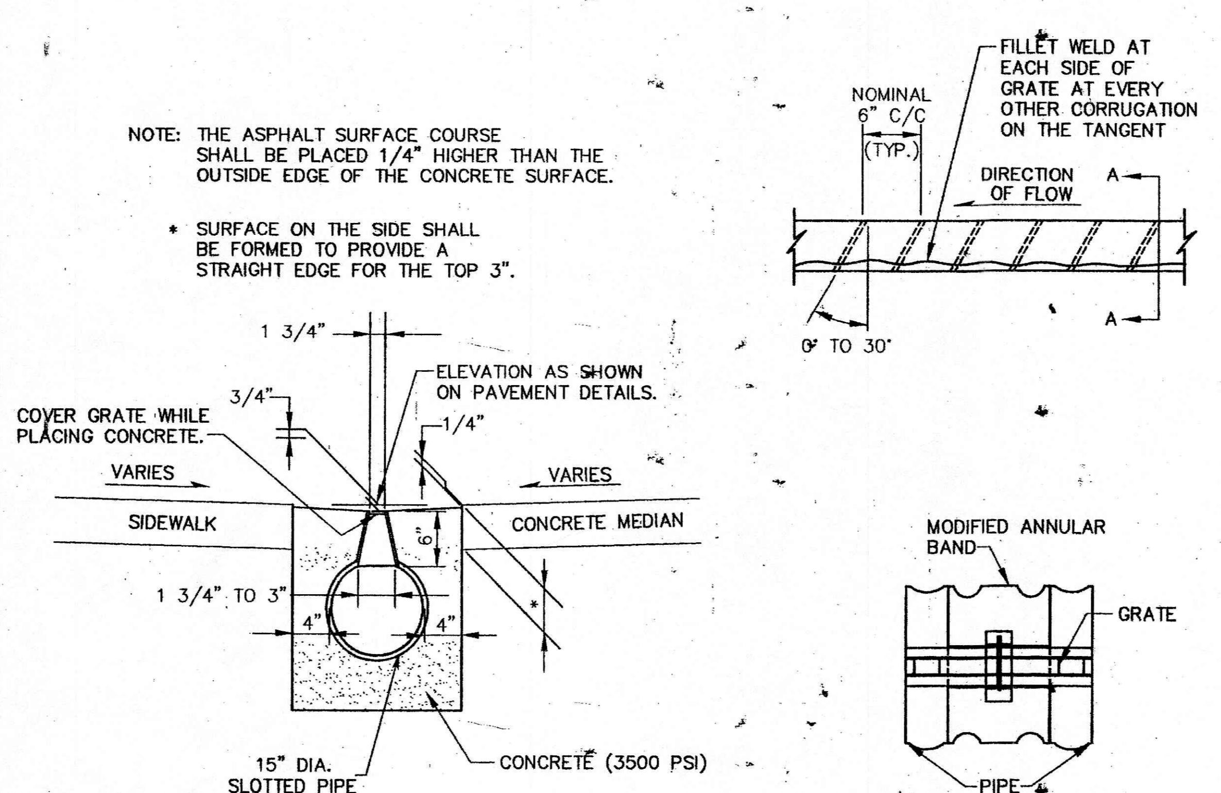
SECTION A-APLAN15" SLOTTED DRAIN, TYPE 2
