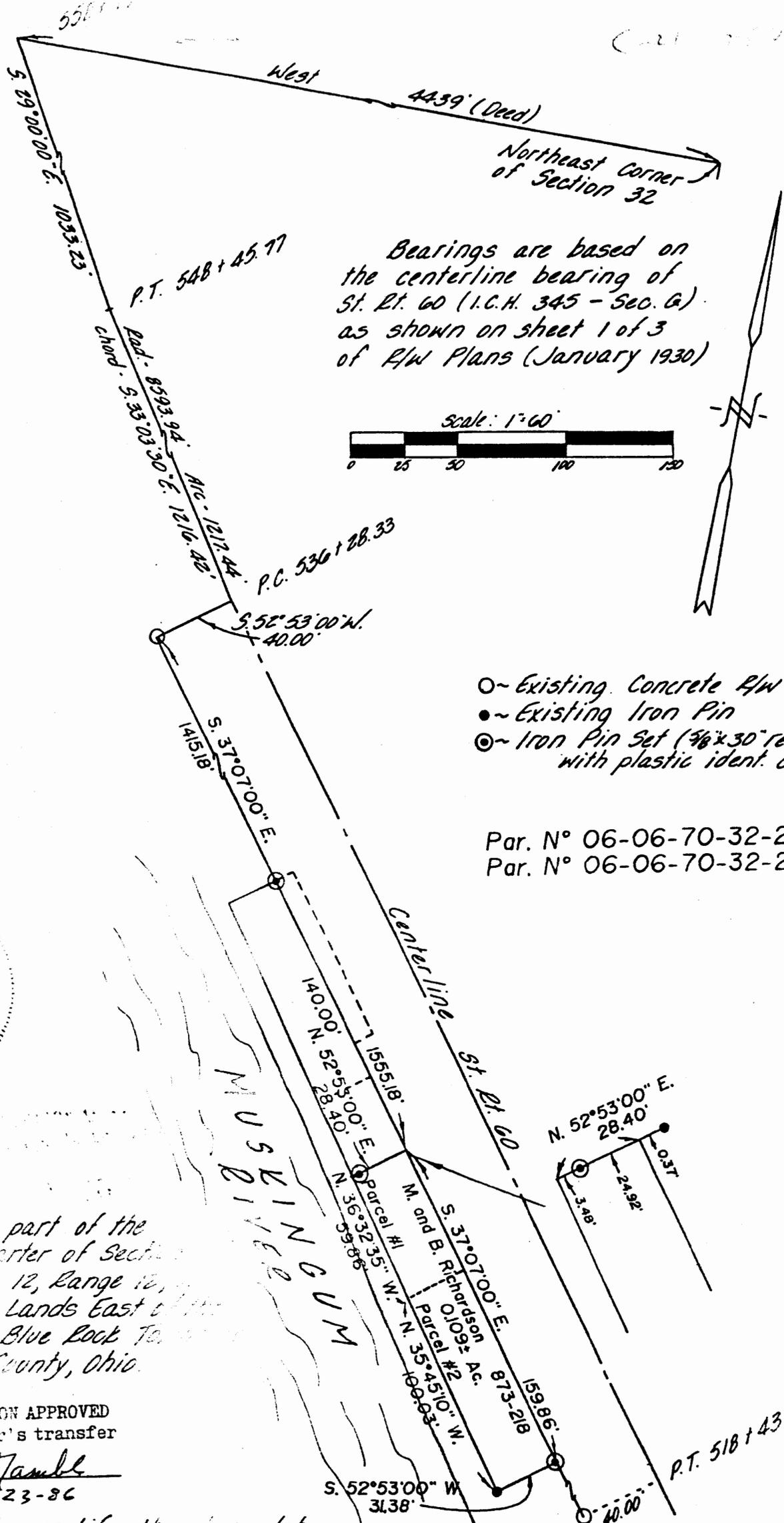
Bearings are based on the centerline bearing of St. Rt. 60 (I.C.H. 345 - Sec. 6) as shown on sheet 1 of 3 of R/W Plans (January 1930)
