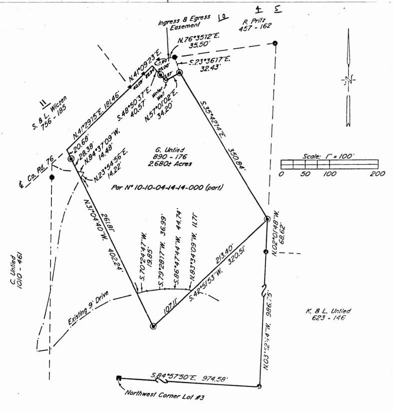
Bearings are based on the centerline of County Road #76 as N.41°29'15"E. as recorded in Vol. 756, Pg. 185 of the Muskingum County Deed Records.
