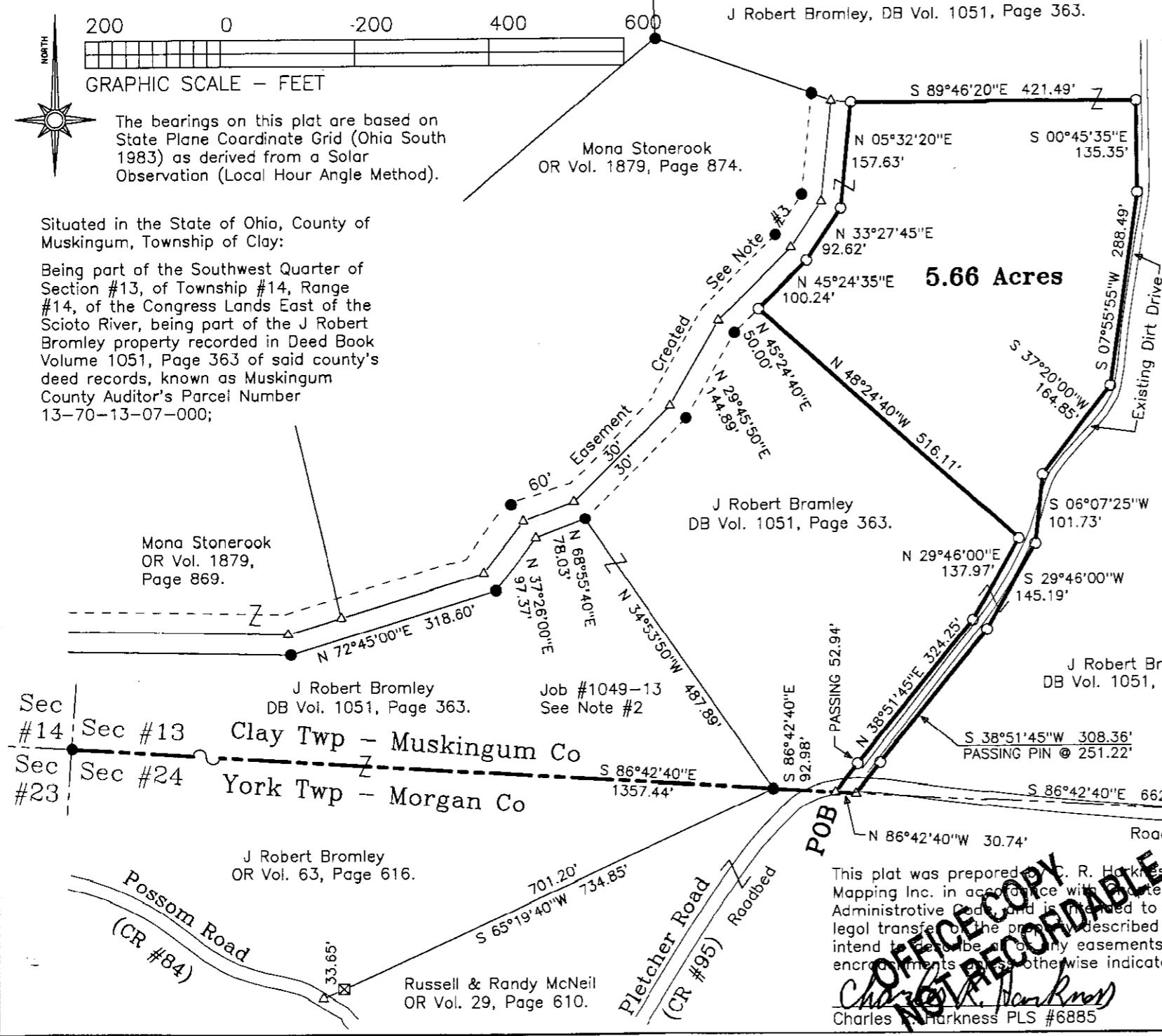
This plat was prepared by Charles R. Harkness Surveying & Mapping Inc. in accordance with Chapter 4733-37 of the Administrative Code, and is intended to be used for the legal transfer of the property described and does not intend to create any easements of record, nor encroachments unless otherwise indicated.
