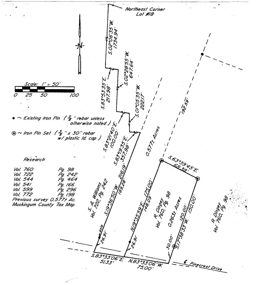
Bearings are based on the deed bearing S.O2°O6'35''W. along the west line of 68,63± Acres (Vol. 760, Pg. 98).
