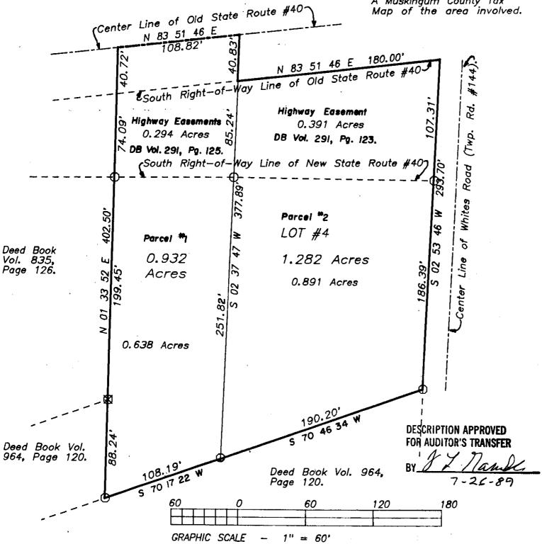
This survey plat was prepared by Charles R. Harkness Registered Surveyor #6885 from an actual survey completed July 25, 1989, and is intended to be used for the legal transfer of the property shown, and does not intend to show all or any easements of record, nor encroachments unless otherwise indicated.
