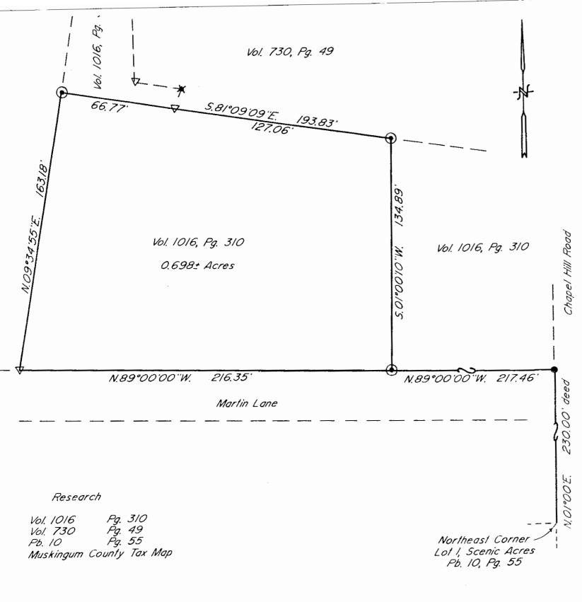
Bearings are based on the South Line of the previous survey of 1.37± Acres as recorded in Vol. 1016, Pg. 310.
