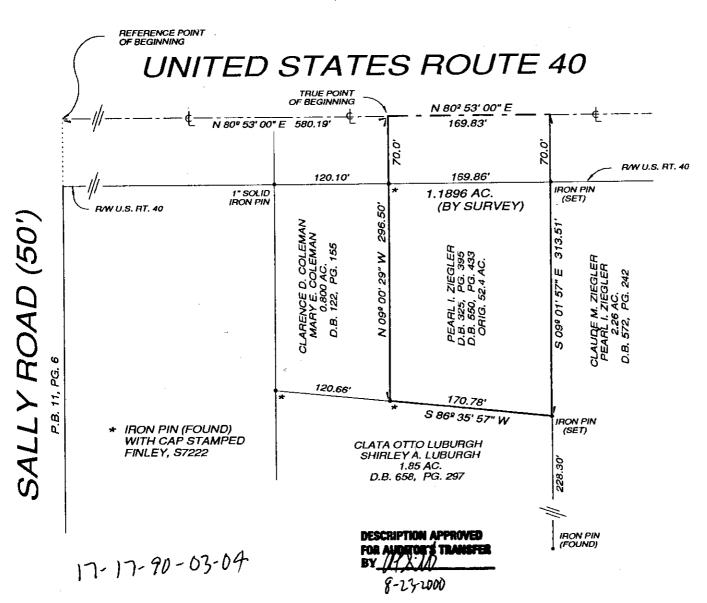
ALL IRON PINS DENOTED AS "SET" ARE 5/8" (I.D.) X 30" IRON PIPE PLUGGED WITH A PLASTIC CAP STAMPED "ELSCO S5519" AND HAVE BEEN SET BY ERLENBACH LAND SURVEYING COMPANY. ALL MONUMENTATION DENOTED AS "FOUND" HAS BEEN SET BY OTHERS.
