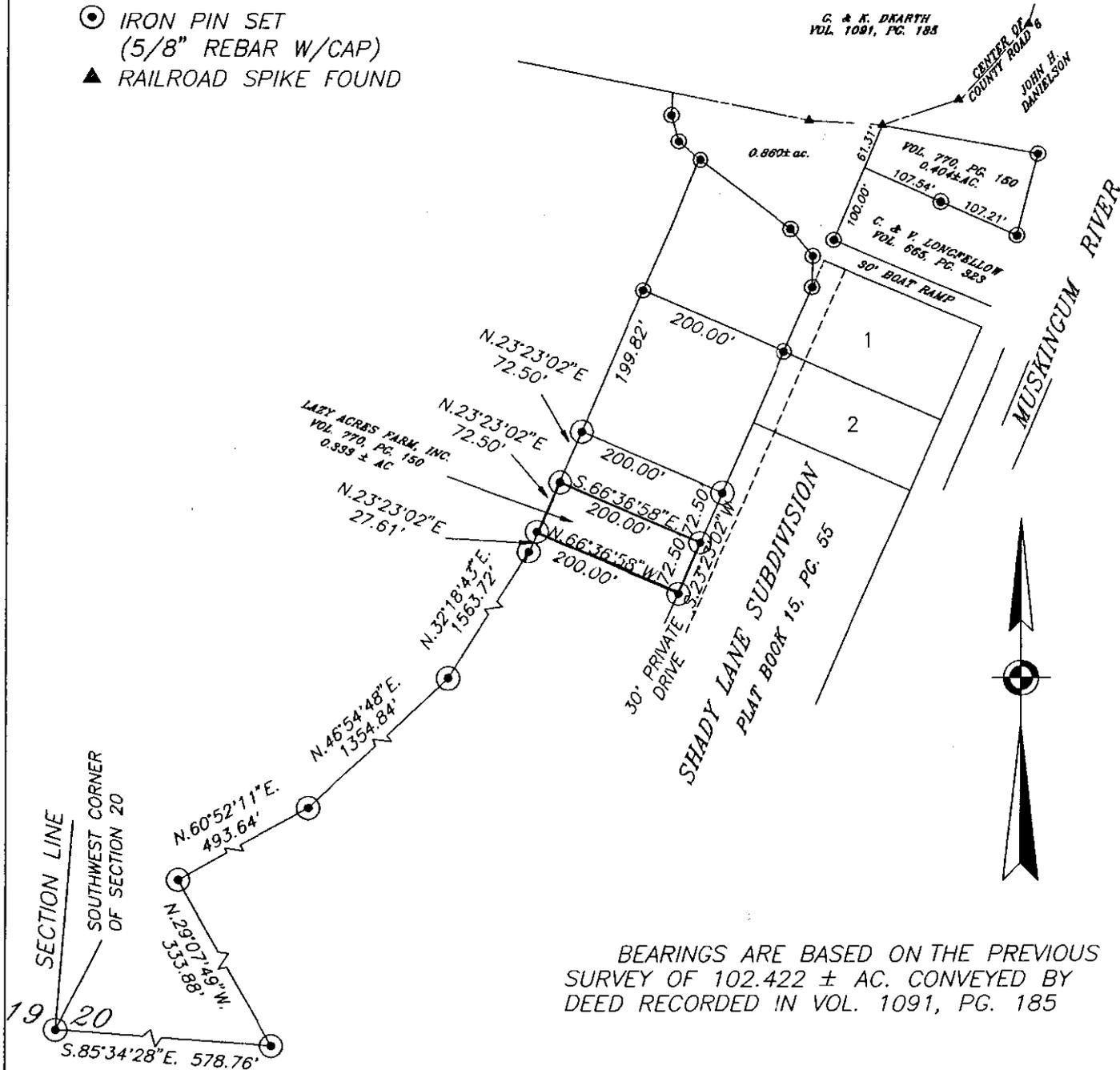
BEARINGS ARE BASED ON THE PREVIOUS SURVEY OF 102.422 ± AC. CONVEYED BY DEED RECORDED IN VOL. 1091, PG. 185
