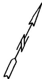
THE BEARINGS OF THIS PLAT ARE BASED ON THE NORTH LINE OF SECTION 16 AS N 90°00'00" W.
