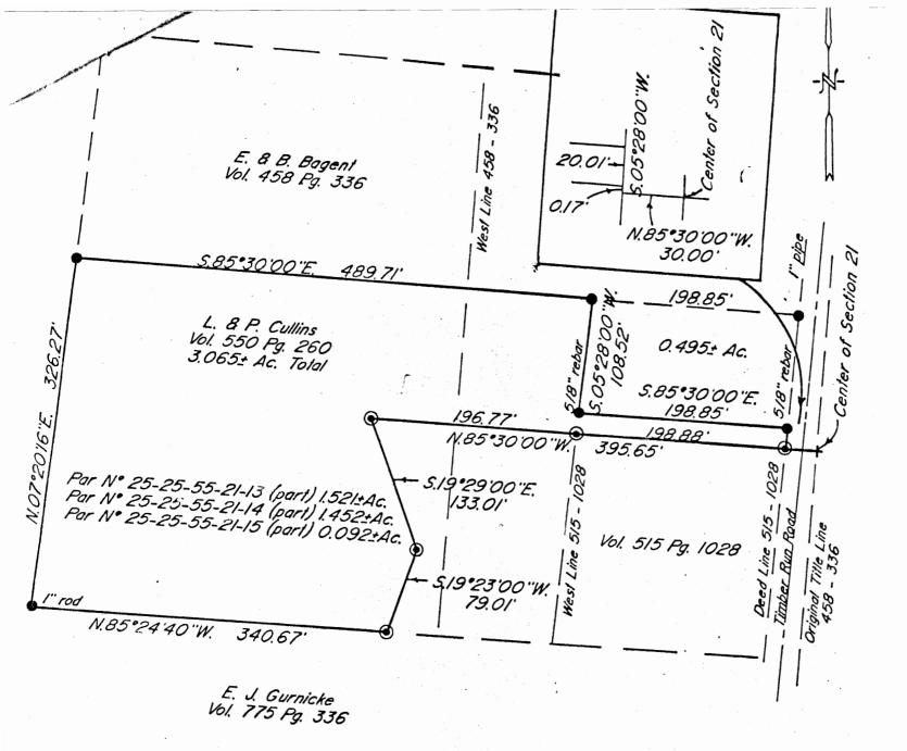
Bearings are based on the deed bearing (N.85°30'W.) on the north line of D.B. Vol. 515, Pg. 1028.
