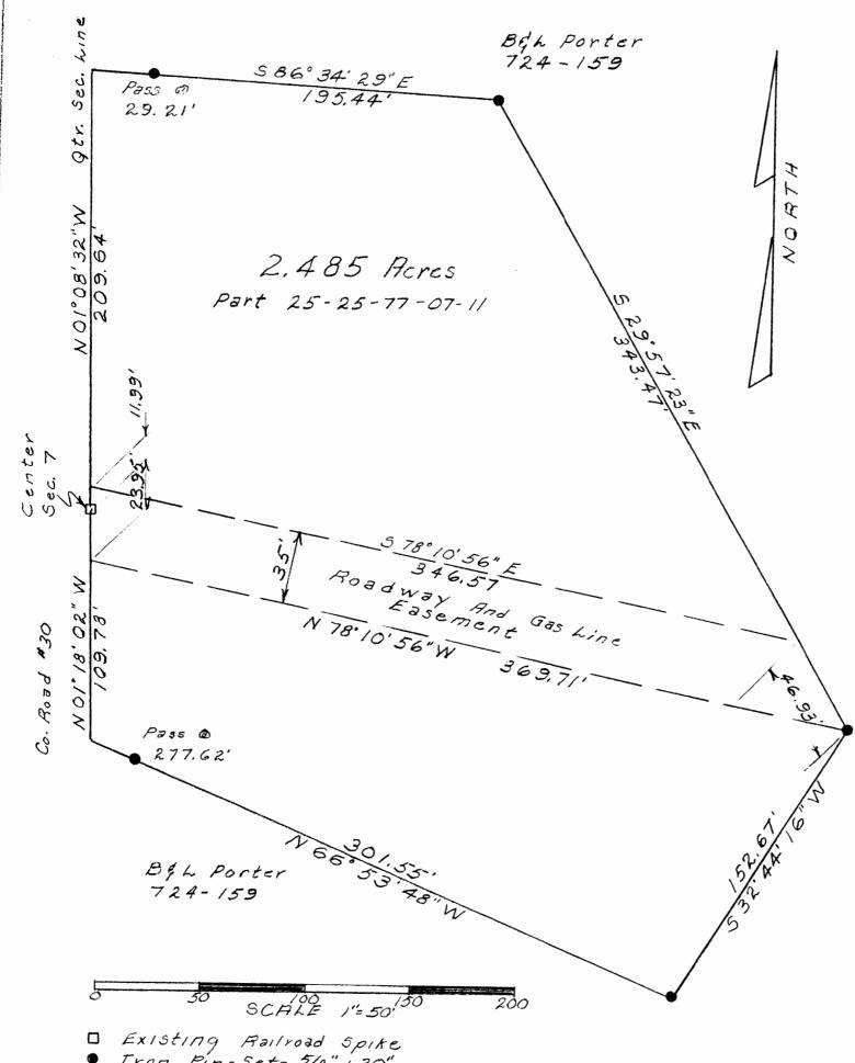
● Iron Pin-Set- 5/8" x 30" Re-bar With Identification Cap
