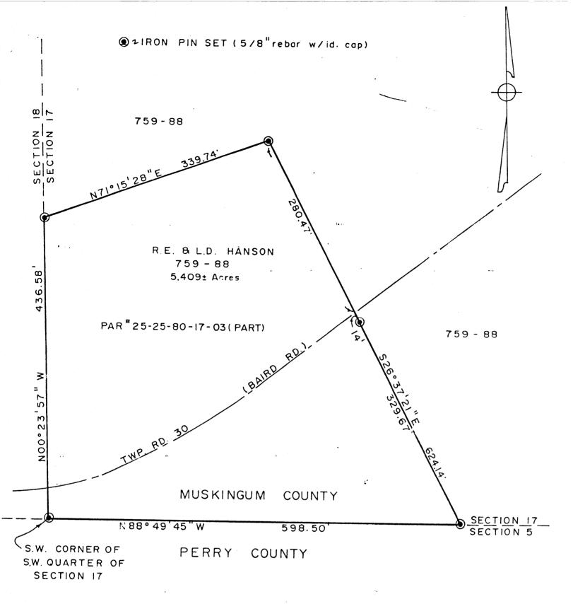
BEARINGS ARE BASED ON AN ASSUMED BEARING OF N88°49'45"W ALONG THE SOUTH LINE OF THE SOUTHWEST QUARTER OF SECTION 17.
