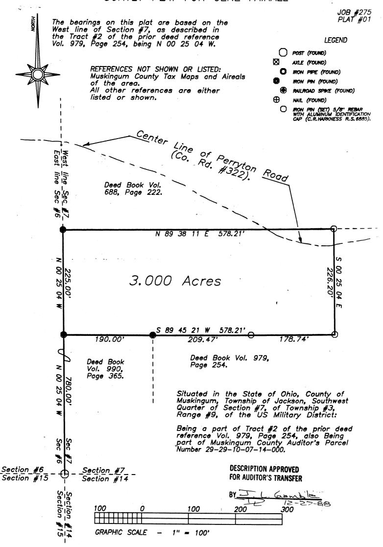
This survey plat was prepared by Charles R. Harkness Registered Surveyor #6885 from an actual survey completed December 16, 1988, and is intended to be used for the legal transfer of the property shown, and does not intend to show all or any easements of record, nor encroachments unless otherwise indicated.
