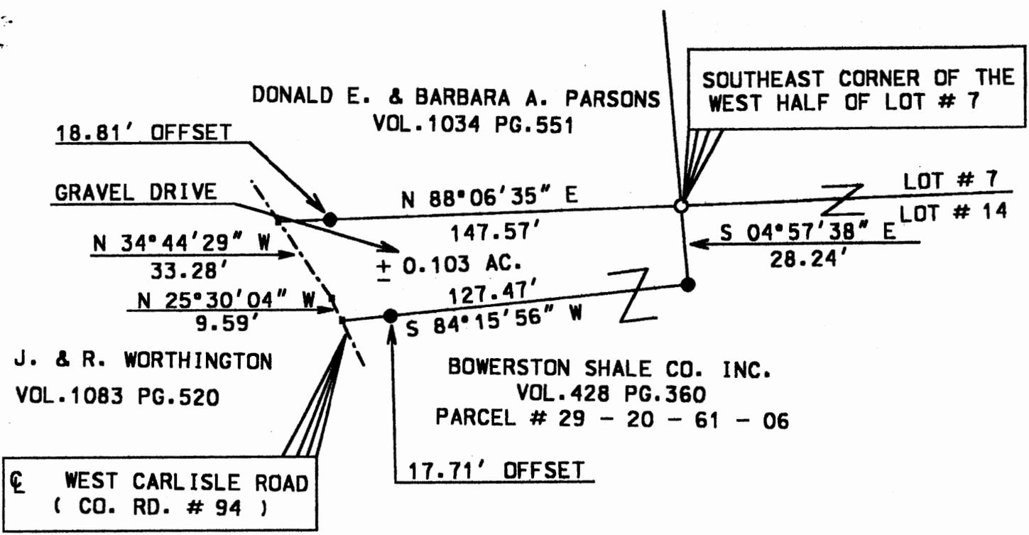
**BASIS OF BEARING :** BEARINGS ON THIS PLAT ARE ASSUMED ON THE SOUTH LINE OF LOT # 7 AS BEING N 88°06'35" E AND ARE FOR ANGULAR CALCATION ONLY.
