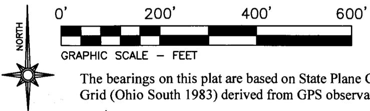
The bearings on this plat are based on State Plane Coordinate Grid (Ohio South 1983) derived from GPS observations.
