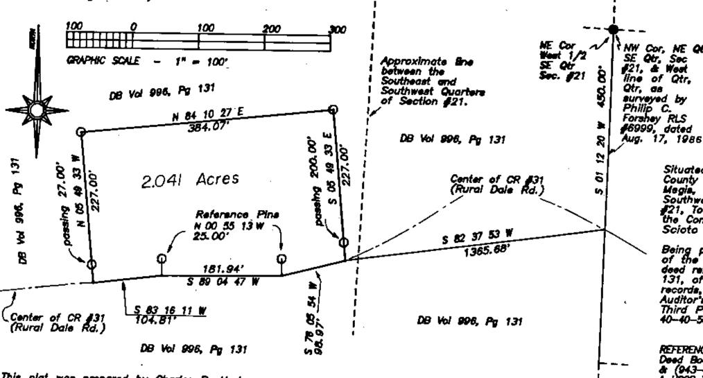
This plat was prepared by Charles R. Harlaness Registered Surveyor #6885 from an actual survey completed on August 1, 1990. This survey is intended to be used for the legal transfer of the property shown, and does not intend to show all or any easements of record, nor encroachments unless otherwise indicated.
