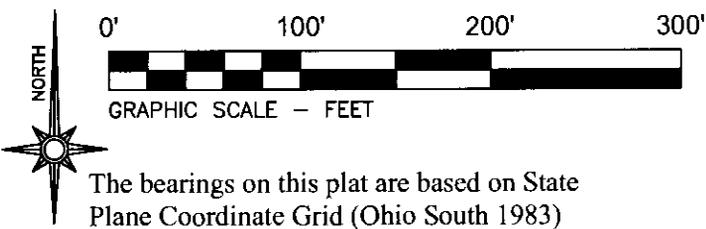
The bearings on this plat are based on State Plane Coordinate Grid (Ohio South 1983) derived from GPS observations.
