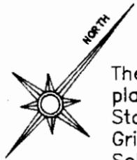
The bearings on this plat are based on State Plane Coordinate Grid derived from a Solar Observation (Local Hour Angle Method).
