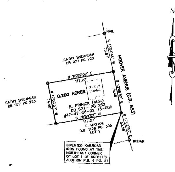
BEARINGS ARE BASED ON THE NORTH LINE OF LOT 1 OF KROFFT'S ADDITION AS BEING S 78'59'02" W AND ARE USED TO DENOTE ANGLES ONLY.
