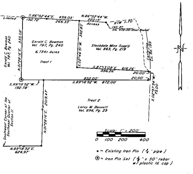
Bearings are based on the Location Plan of I-70 as recorded in Pb. II, Pg. 20 of the Muskingum County Plat Records.
