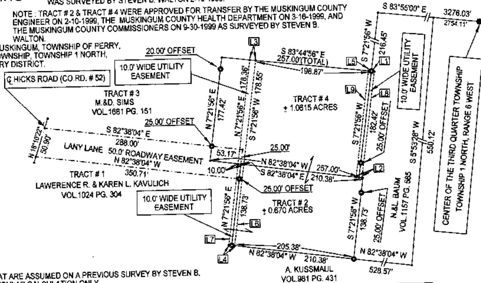
BASIS OF BEARING : BEARINGS ON THIS PLAT ARE ASSUMED ON A PREVIOUS SURVEY BY STEVEN B. WALTON DATED 2-10-1999, AND ARE FOR ANGULAR CALCULATION ONLY.
