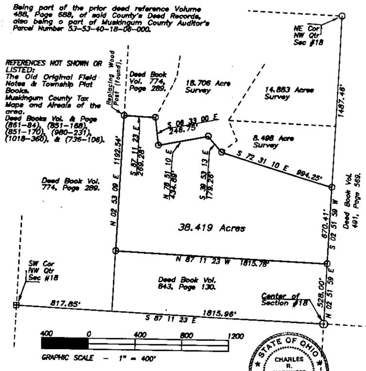
This survey plat was prepared by Charles R. Harkness Registered Surveyor \$6885 from an actual survey completed July 18, 1989, and is intended to be used for the legal transfer of the property shown, and does not intend to show all or any sacements of record, nor encroachments unless otherwise indicated.
