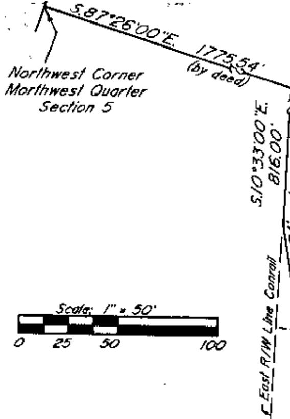
Bearings are based on the Bearing of S.10°33'00\"/>
