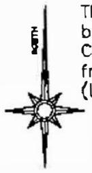
The bearings on this plot are based on State Plane Coordinate Grid as derived from a Solar Observation (Local Hour Angle Method).
