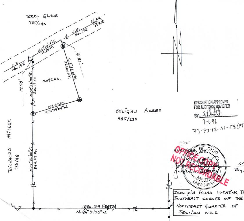
LEGEND: - I FON PINS OR PIPES FOUND \* - EXISTING FENCE LINE - - IRON PINS SET ARE ONE HALF INCH REBAR 30 INCHES LONG WITH IDENTIFICATION CAPS. (J.LE. P.S. 6410). - THE BEATINGS FOR THIS SURVEY AR BASED ON THE SOUTH LINE OF THE NORTHE QUARTER OF SECTION NO. 2 AS BEING NORTH B6°31'00" WEST. IR- PROPERTY LINE DATA REFERENCES: TAX MAPS, USGS MAP, DEEDS OF RELORD. VOL. 985, P. 230 VOL. 755, P. 243 " 926, P. 48 " 1006, " 575 " 985, " 228 SURVEYS BY - LOREN CAMP.
