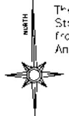
The bearings on this plat are based on State Plane Coordinate Grid as derived from a Solar Observation (Local hour Angle Method).
