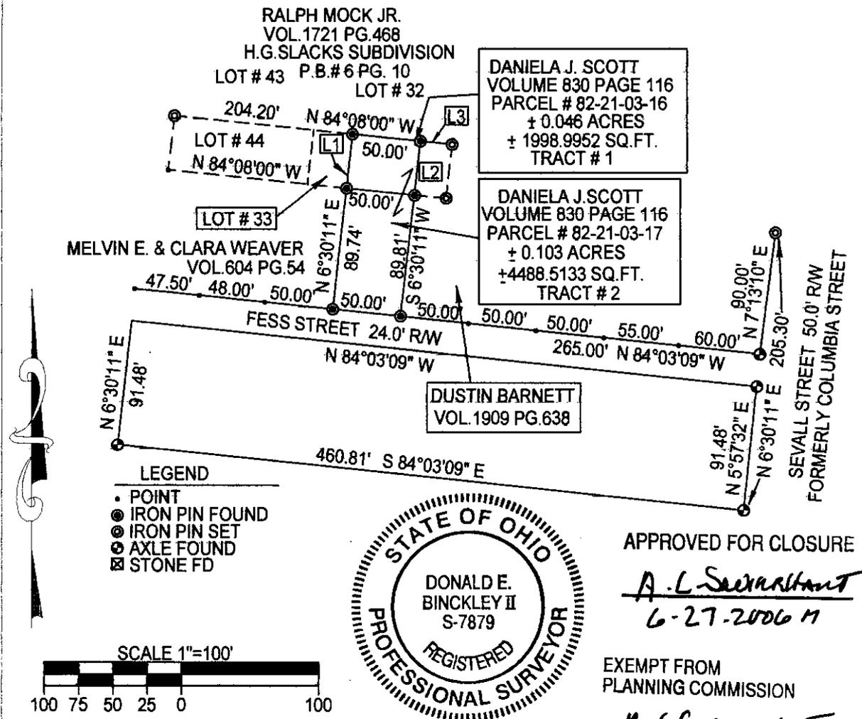
BASIS OF BEARING : BEARINGS ON THIS PLAT ARE BASED ON A PREVIOUS SURVEY OF LOT # 43 AND LOT # 32 OF H.G. SLACK'S SUBDIVISION P.B.#6, PG.10 BY MAX GRAVES DATED 11-10-1999 AND ASSUME THE SOUTH LINE OF LOT # 32 AND LOT # 43 AS BEING NORTH 84 DEGREES 08 MINUTES 00 SECONDS WEST AND ARE FOR ANGULAR CALCULATION ONLY.
