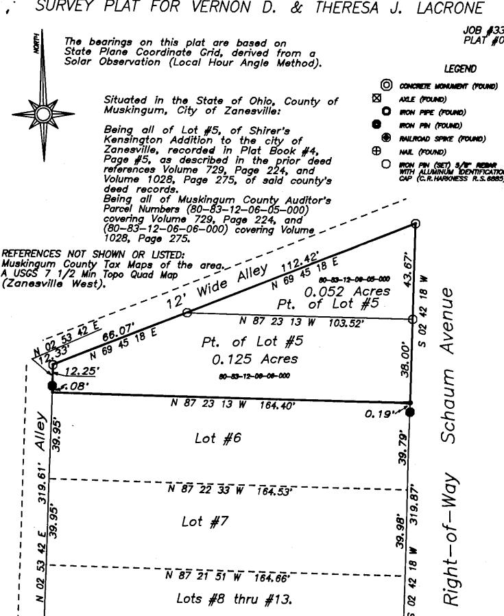
NOTE -Proration of Lot demensions was accomplished by re—establishing the Block, with existing curbs, and subsequent survey information.
