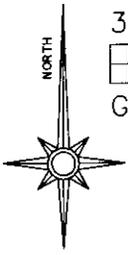
The bearings on this plat are based on State Plane Coordinate Grid (Ohio South 1983) as derived from a Solar Observation (Local Hour Angle Method).
