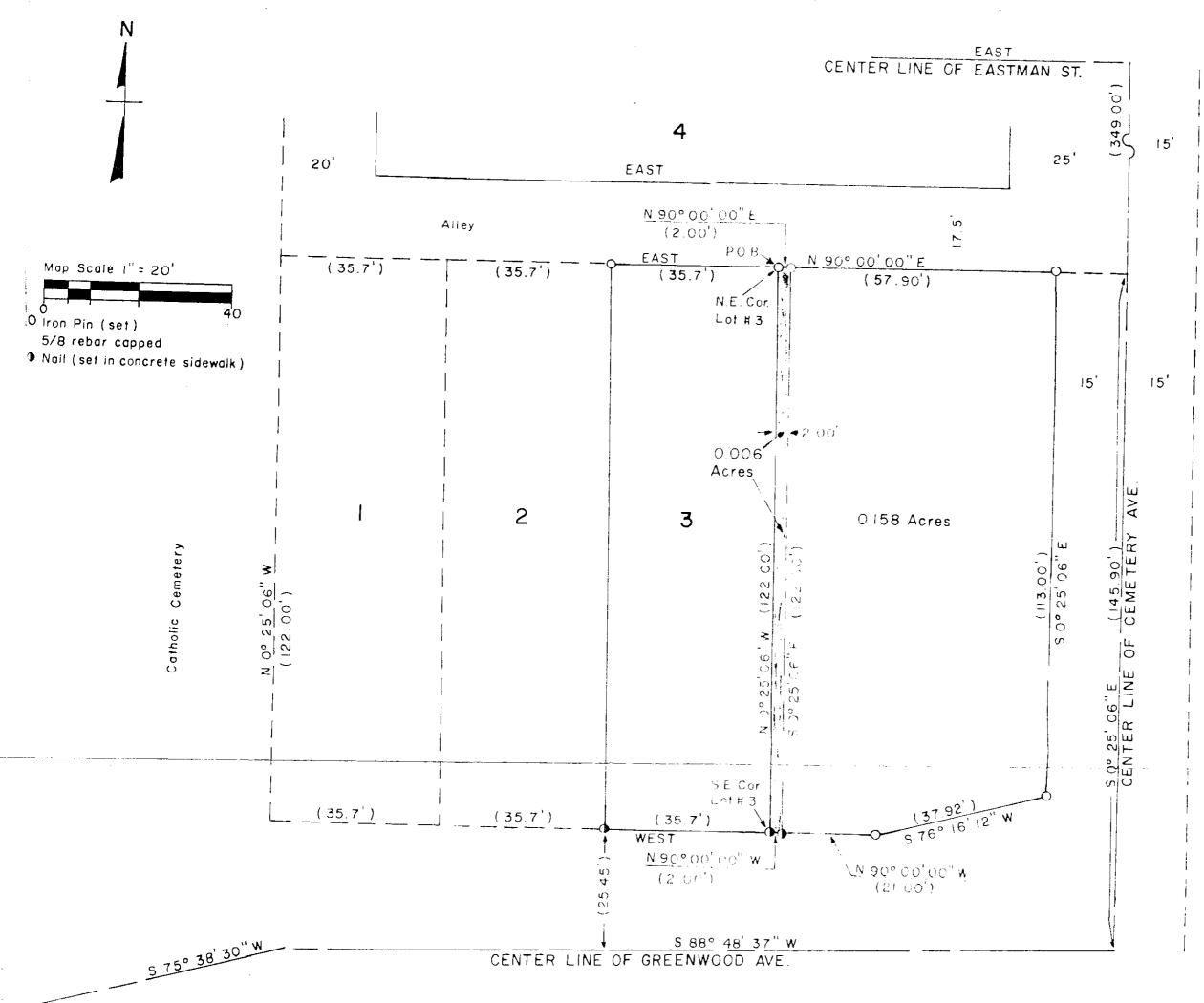
Basis For Bearings on this Plat the Center Line of Eastman St. which was given an arbitrary Bearing of Due East
