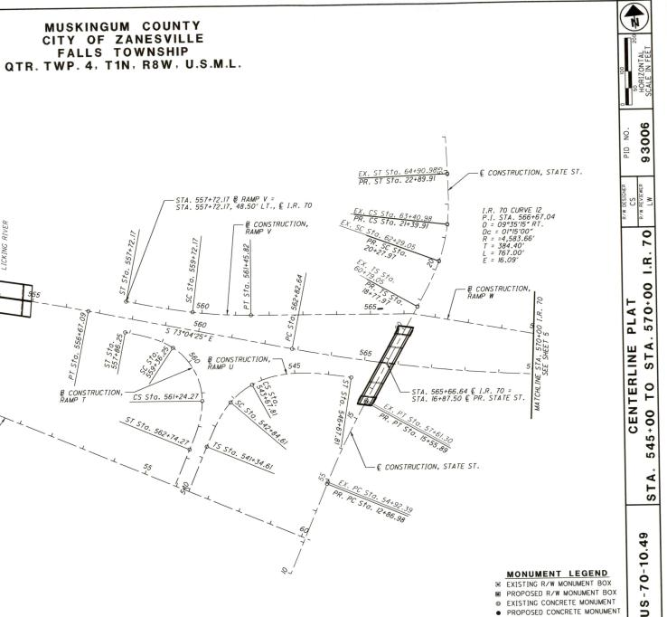
SETTING OF ALL MONUMENTS SHALL BE PERFORMED BY A SURVEYOR REGISTERED IN THE STATE OF OHIO. THE MONUMENT ASSEMBLIES AND REFERENCE MONUMENTS WILL BE INSTALLED BY THE CONTRACTOR AT THE TIME OF CONSTRUCTION. THE IRON PIN AND CAP (WHEN REQUIRED) ARE TO BE INSTALLED BY THE CONTRACTOR'S SIDVEYOR CONTRACTOR'S SURVEYOR.
