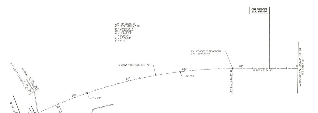
SETTING OF ALL MONUMENTS SHALL BE PERFORMED BY A SURVEYOR REGISTERED IN THE STATE OF OHIO. THE MONUMENT ASSEMBLIES AND REFERENCE MONUMENTS WILL BE INSTALLED BY THE CONTRACTOR AT THE TIME OF CONSTRUCTION. THE IRON PIN AND CAP WHEN REQUIRED) ARE TO BE INSTALLED BY THE CONTRACTOR'S SURVEYOR.
