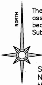
The bearing on this plat are based on an assumed bearing approximating the bearing as shown on the Plat of Garrett's Subdivision
