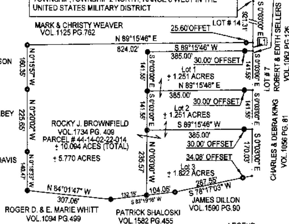
BASIS OF BEARING: BEARINGS ON THIS PLAT ARE ASSUMED ON THE EAST LINE OF LOT # 14 AS SURVEY BY J. G. EPPLEY AS BEING S 00°03'00" E AND ARE ASSUMED FOR ANGULAR CALCULATION ONLY.
