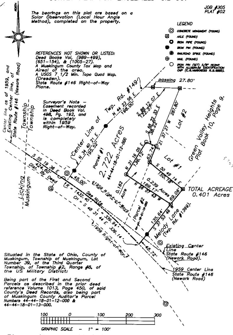
This survey plat was prepared by Charles R. Harkness Registered Surveyor #6885 from an actual survey completed January 24, 1990, and is intended to be used for the legal transfer of the property shown, and does not intend to show all or any easements of record, nar encroachments unless otherwise indicated.
