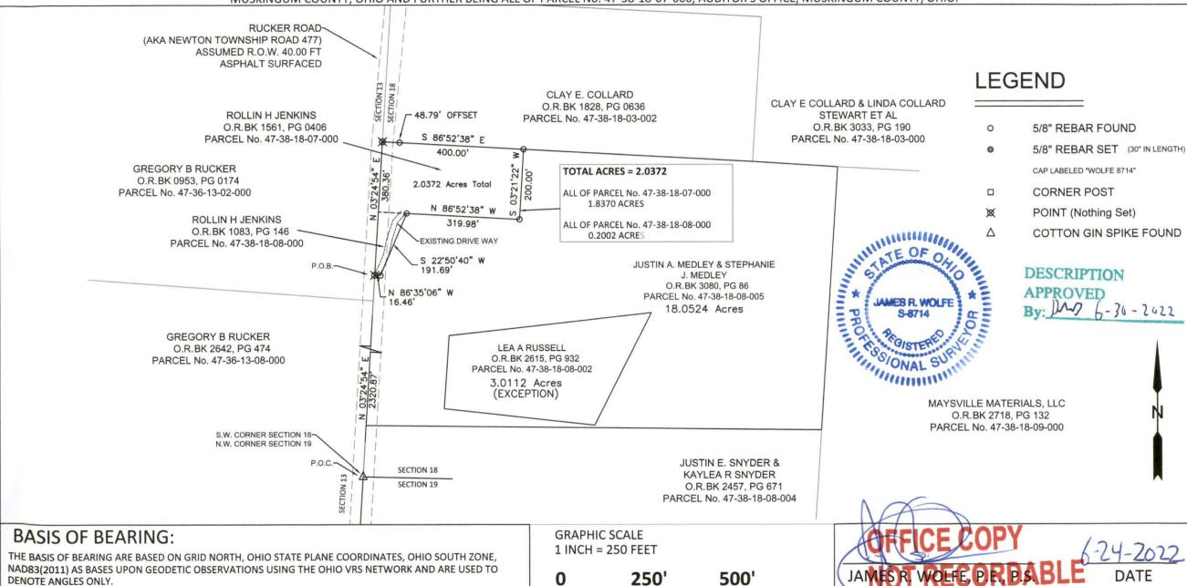
THIS PLAT WAS PREPARED BY JAMES R. WOLFE P.E., P.S., OHIO REGISTERED SURVEYOR NO. 8714, FROM AN ACTUAL FIELD SURVEY PERFORMED IN JUNE 2022 AND FROM DEEDS AND PLATS OF RECORD ON FILE IN THE
