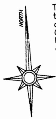
The bearings on this plat are based on a Solar Observation (Local Hour Angle Method) completed on the property.
