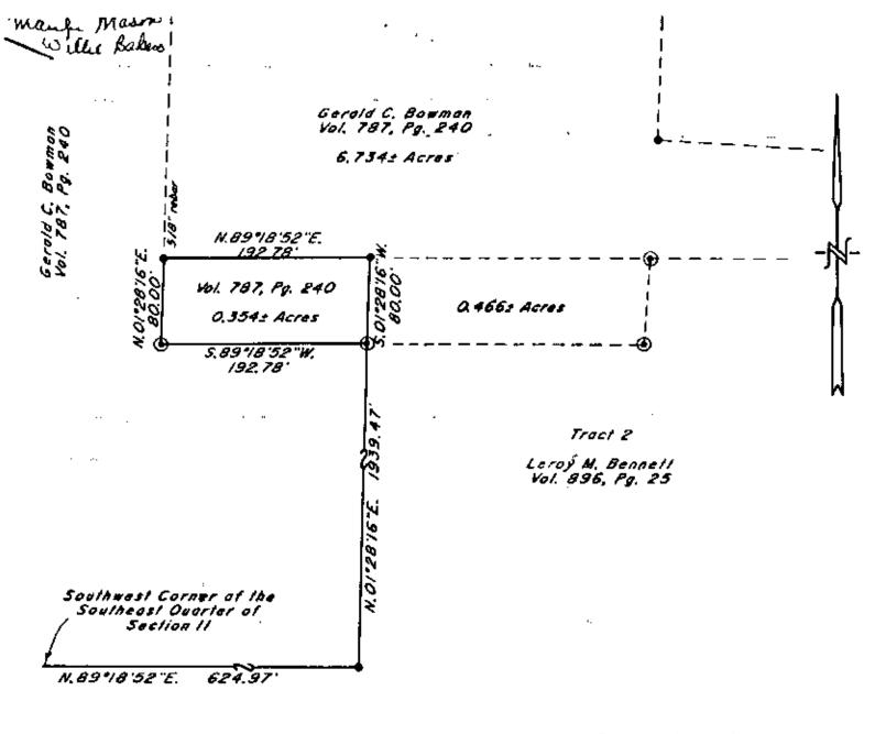
Bearings are based on the Location Plan of I-70 as recorded in Pb. II, Pg. 20 of the Muskingum County Plat Records.
