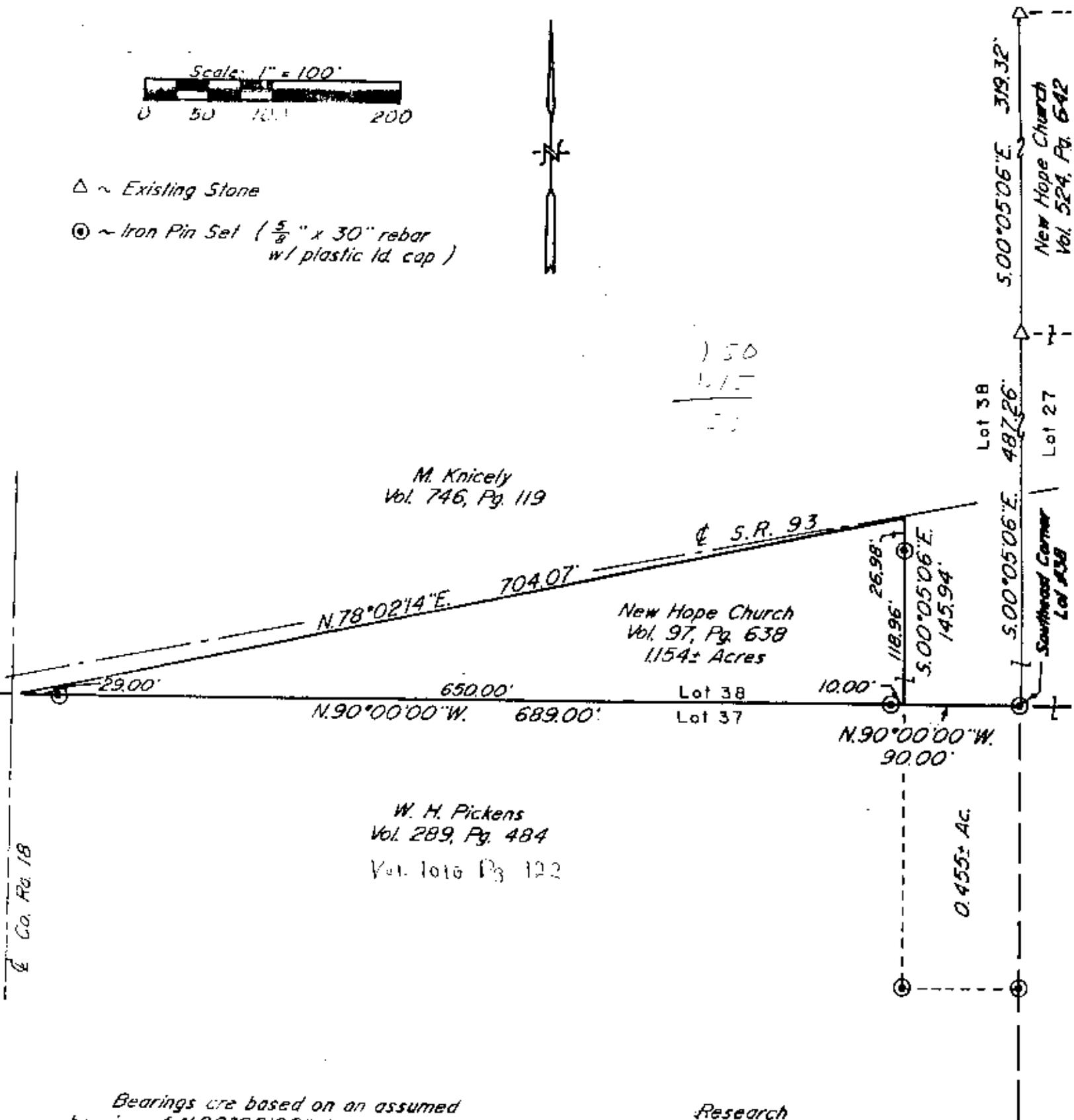
Bearings are based on an assumed bearing of N.90°00'00"W. along the North Line of Lot 37.
