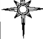
The bearings on this plat are based on State Plane Coordinate Grid as derived from a Solar Observation (Local Hour Angle Method).
