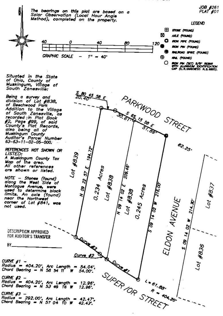
This survey plot was prepared by Charles R. Harkmess Registered Surveyor \$6885 from an octual survey completed NOT Research September 27, 1988, and is intended to be used for the legal transfer of the property shown, and does not intend to show all or any easements of record, nor encroachments unless otherwise indicated.
