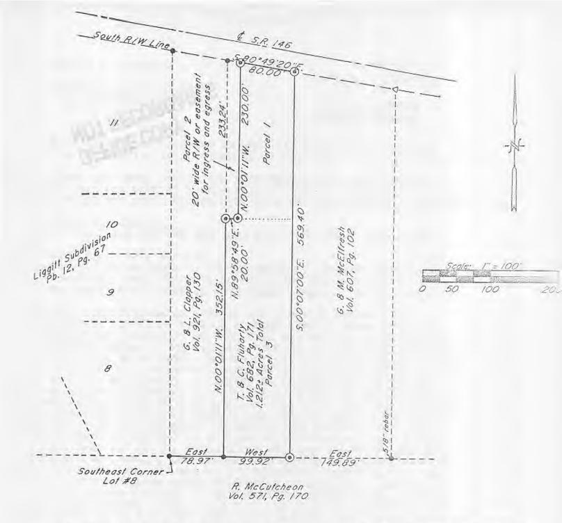
Bearings are based on the west line of the previously surveyed 1.703. Acres as conveyed to G. & L. Clapper as recorded in Deed Vol. 921, Pg. 130 of the Muskingum County Deed Records.
