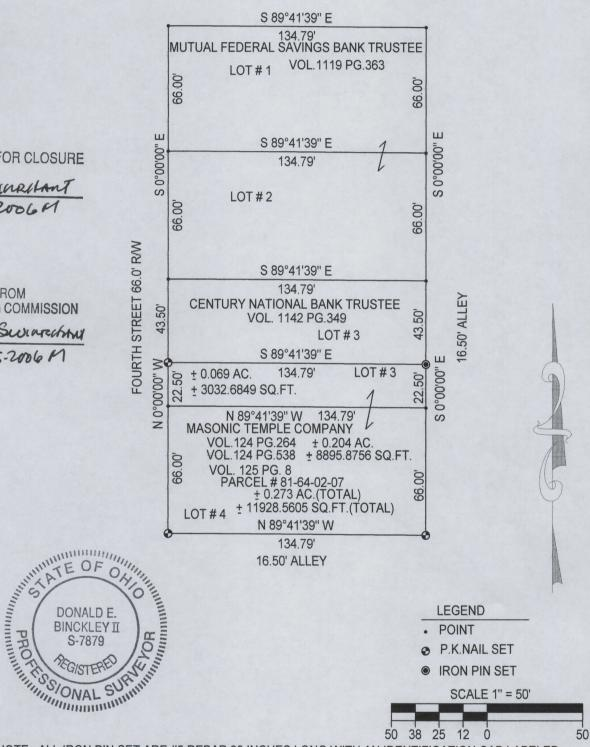
NOTE: ALL IRON PIN SET ARE #5 REBAR 30 INCHES LONG WITH AN IDENTIFICATION CAP LABELED "BINCKLEY S-7879".
