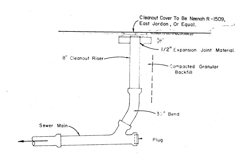
GRAVITY SEWER CLEANOUT DETAIL
