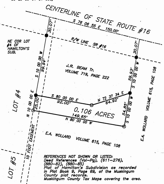
This plat was prepared by Charles R. Harkness Registered Surveyor #6885 from an actual survey completed on April 28, 1988, and is intended to be used for the legal transfer of the property, and deep not intend to show all or any easements of record, no transfer that unless otherwise indicated.
