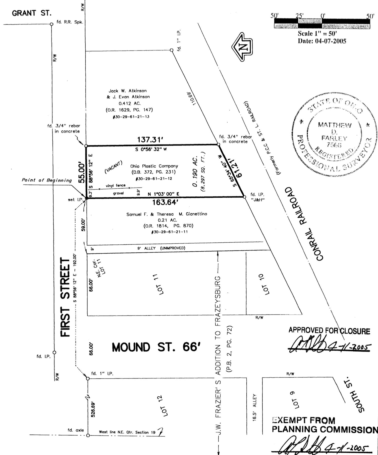
We hereby certify that the foregoing Boundary Survey was prepared from actual field measurements in accordance with Chapter 4733-37 Ohio Administrative Code. Iron pipes set are 30"x1" O.D. with an orange plastic plug inscribed "P.S. 6579", unless otherwise noted. Bearings are based on the centerline of Second Street held as South 62 41' 00" East.
