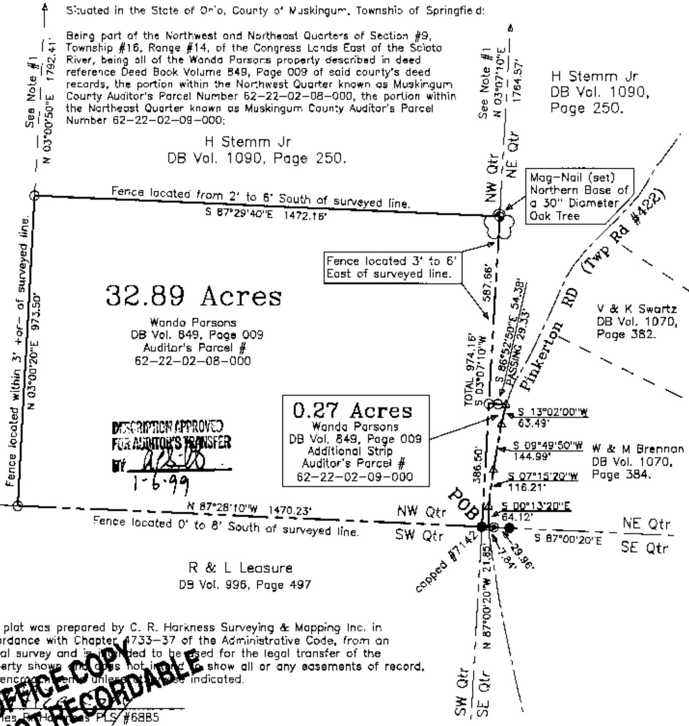
This plat was prepared by C. R. Harkness Surveying & Mapping Inc. in accordance with Chapter 4733-37 of the Administrative Code, from an actual survey and is intended to be used for the legal transfer of the property shown. It does not intend to show all or any easements of record, nor encroachments, unless otherwise indicated.
